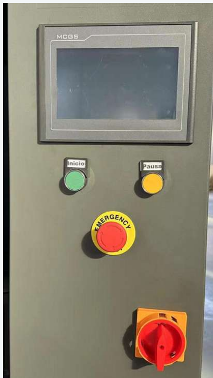
Control detail | Screen, controls and emergency stop
